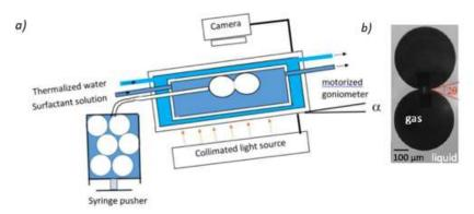
a) Side view of two bubbles immersed in a surfactant solution, confined under a transparent plate inclined by an angle α.
