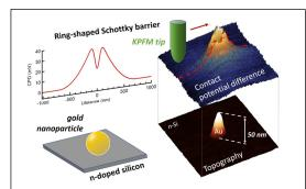
Fig. 1. Measure with Kelvin Probe Force Microscopy (KPFM) of the local electric field generated by a nanoscale Schottky barrier, made of a 50 nm gold nanoparticle on silicon ([Ref 2]. <u>Upper images</u>: electric potential profile. <u>Lower images</u>:
