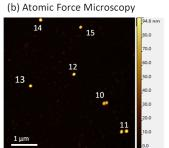
Fig. 1. (a) Dark field optical microscopy image showing several single or dual gold nanoparticles of size 90 mn (b) The same area observed with AFM. Both images are of size 5  $\mu$ m x 5  $\mu$ m [Ref 3]
